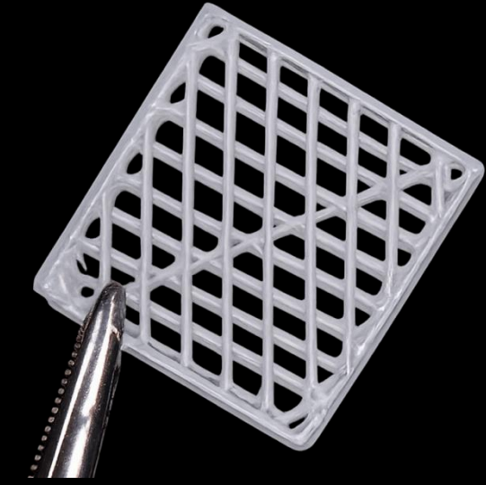
Fig1: 36 PCL Group: Osteopore® custom-printed scaffolds (75% PCL / 25% \beta -TCP).
