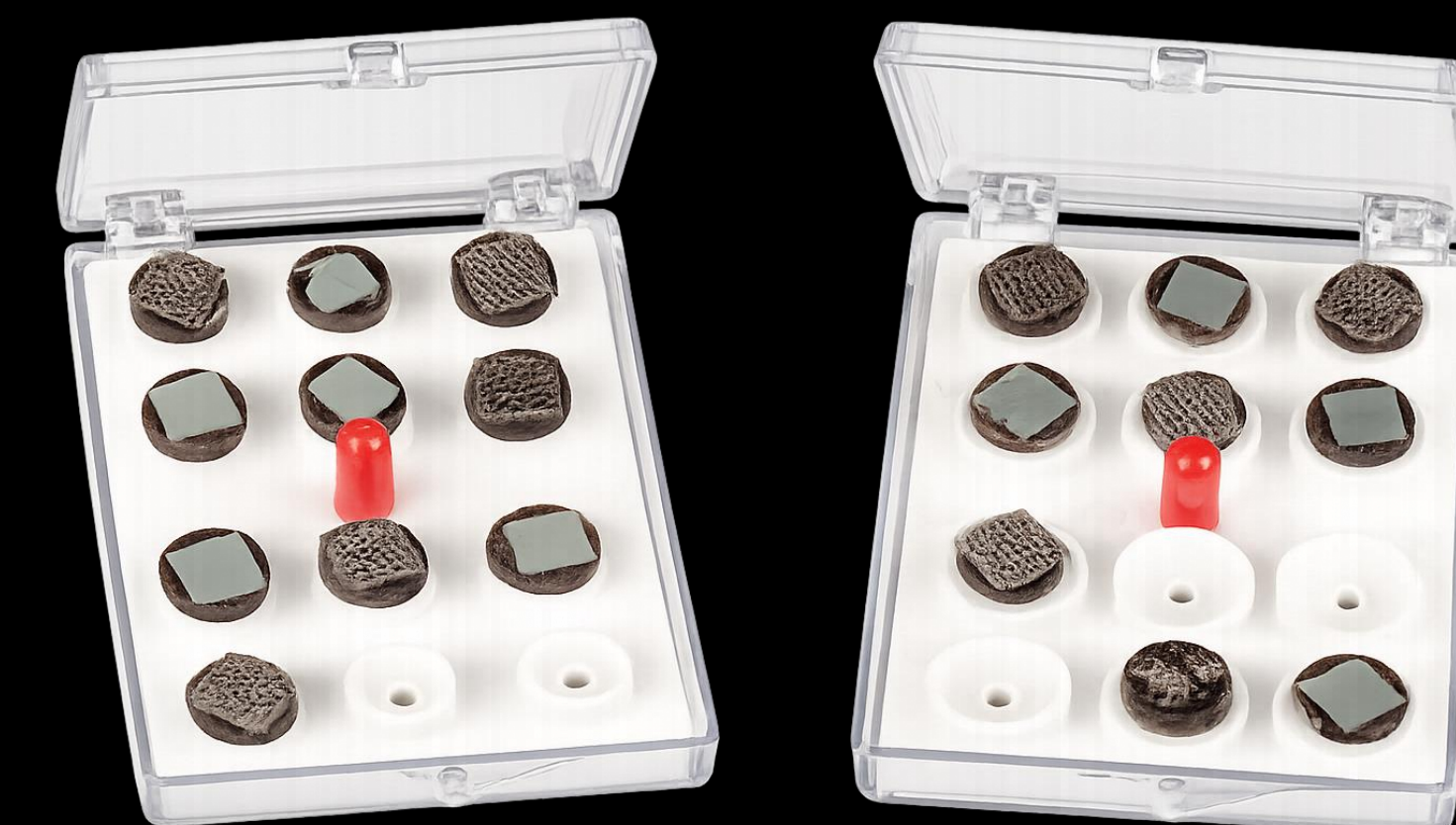
Fig8: Specimen mounting setup used for SEM preparation.
